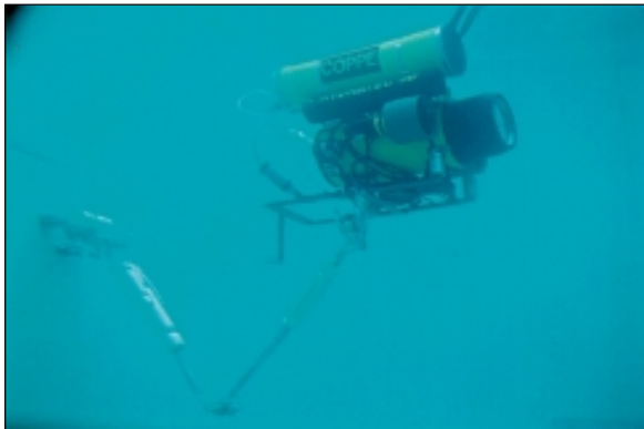
Figure 3. The passive arm installed on the MKII ROV.
