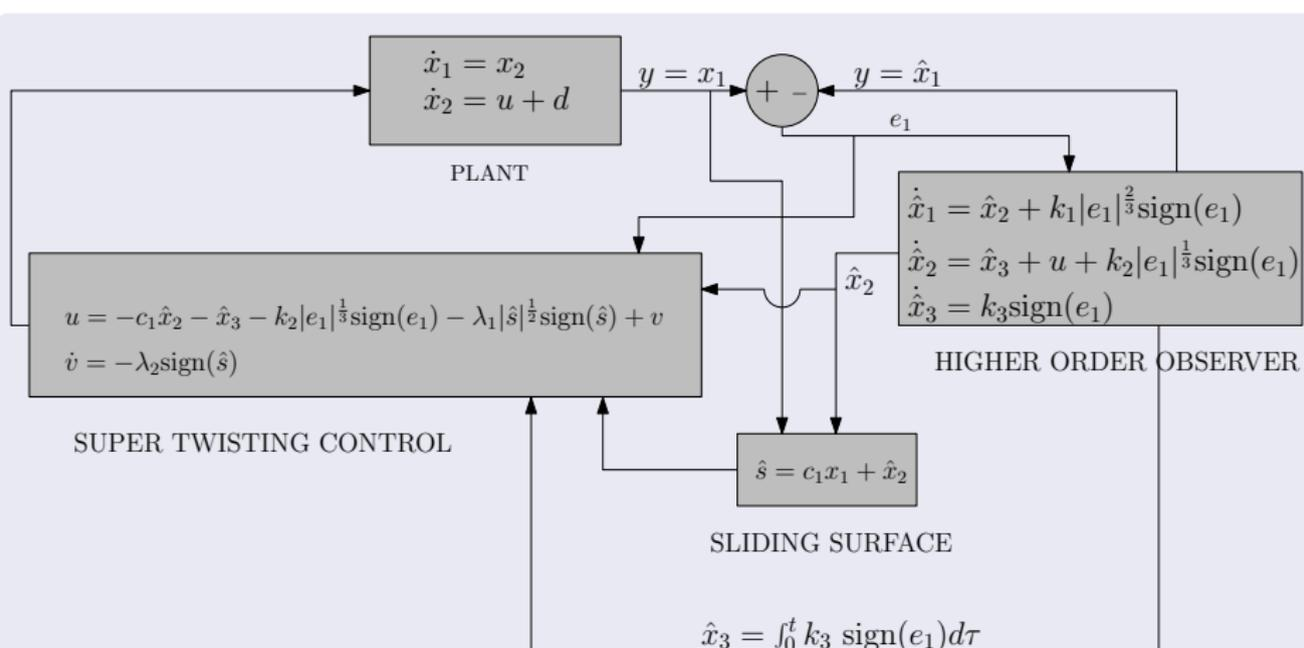
**Figure:** Block diagram of the Super Twisting Control based on HOSM Observer
