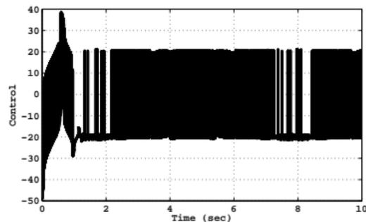
Figure: Discontinuous Integral Sliding Mode Control with disturbance.
