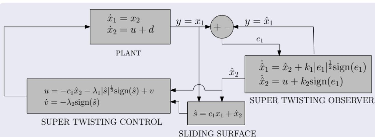
**Figure:** Block diagram of the Super Twisting Control based on Super Twisting Observer
