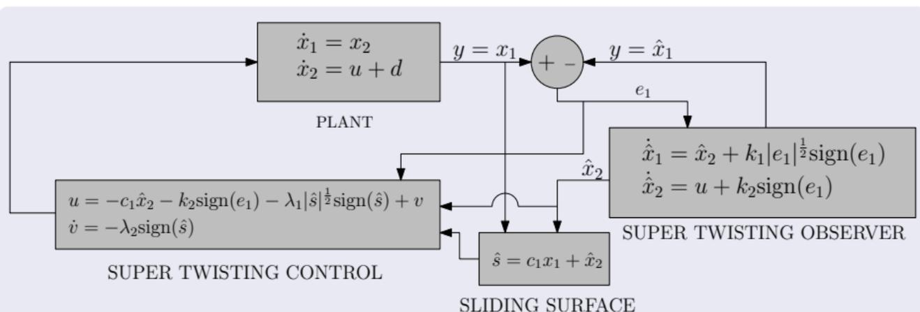
Figure: Block diagram of the Proposition 1 control based on Super Twisting Observer
