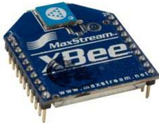
Figura 20: Antena Chip.
