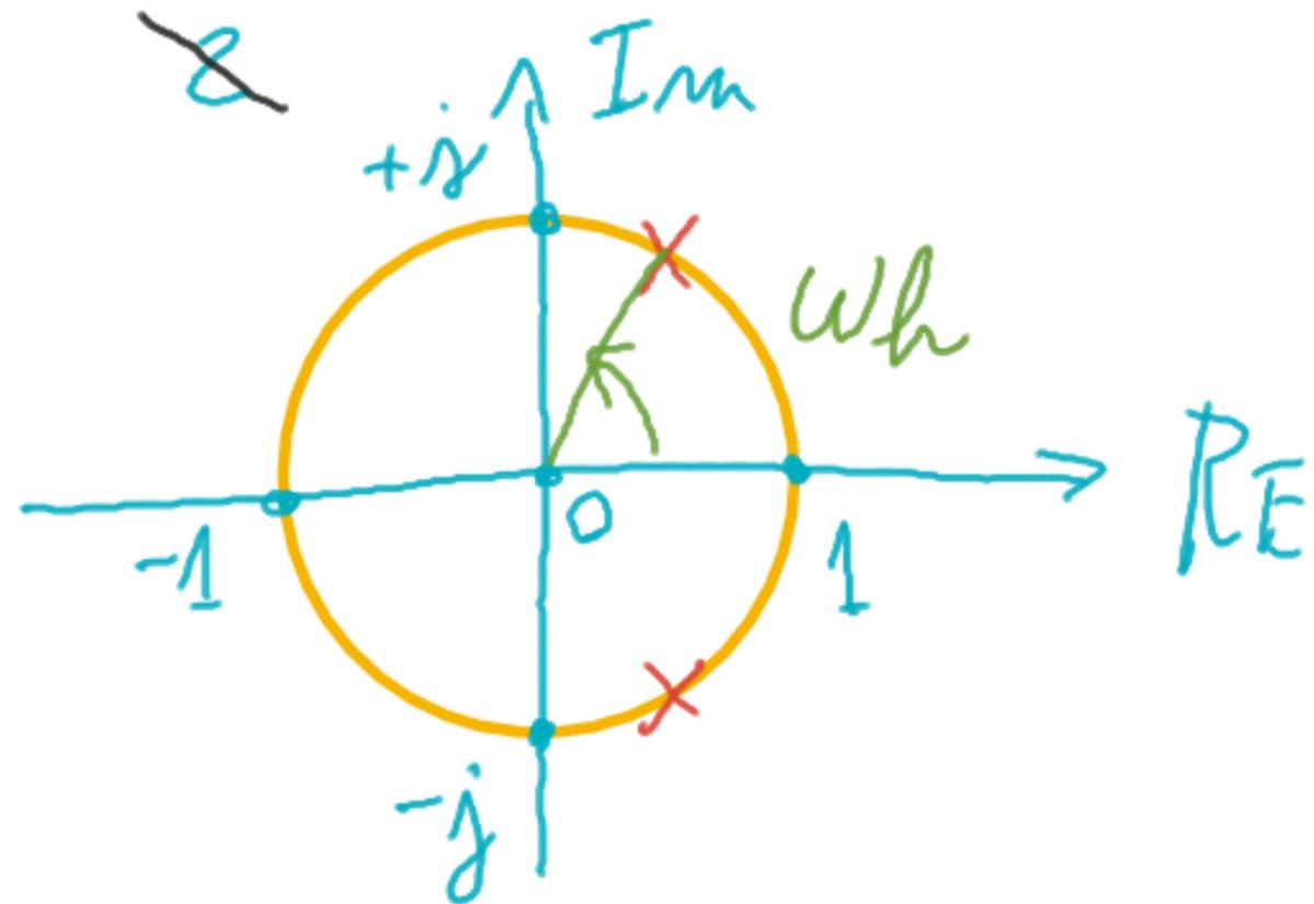
$$\Phi = \begin{bmatrix} \cos \omega h & \sin \omega h \\ -\sin \omega h & \cos \omega h \end{bmatrix}$$
