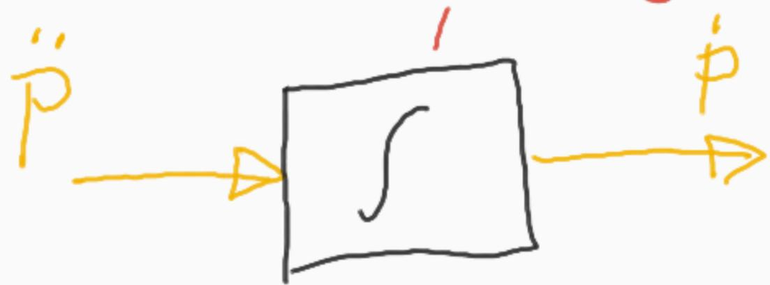
$$\dot{p}(t) = \int \ddot{p}(t) dt = \int a dt = at + v_0$$
